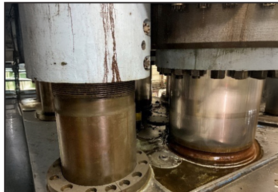
Leakage around rams was evident.
