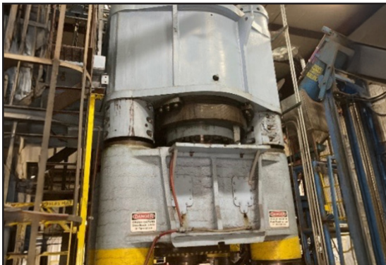
5,000-ton compaction press was too large to disassemble.
